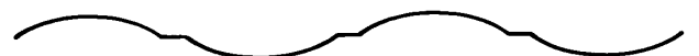
Fig. 28B — Smaller Amplitude Sine Wave with same amount (higher %) of Crossover (notch) Distortion.
